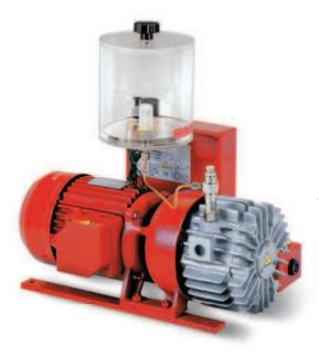
These vacuum pumps having a suction capacity of 10, 15 and 20 cum/h. The vacuum lubrication with oil recirculation can be adjusted via an oiler located in correspondence of the suction inlet.
