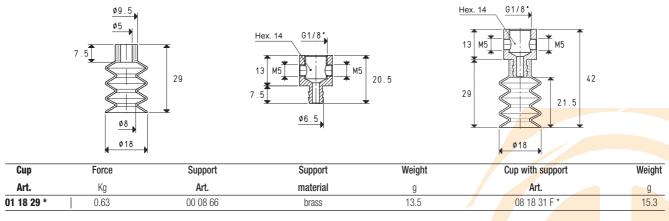
$<sup>^{\</sup>star}$  Complete the code indicating the compound: A= oil-resistant rubber; N= natural para rubber; S= silicon
