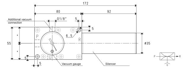
P=COMPRESSED AIR CONNECTION R=EXHAUST U=VACUUM CONNECTION
