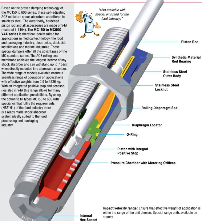
Material: Shock Absorber body and locknut: Stainless steel (1.4404/ AISI 316L). Piston rod: Hardened stainless steel (1.4125/AISI 440C). Rolling diaphragm seal: EPDM. Accessories: Stainless steel (1.4404/ AISI 316L).
